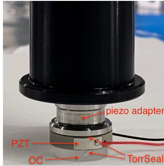
Fig. 3.11 The assembly of piezo to output coupler using TorrSeal glue.
